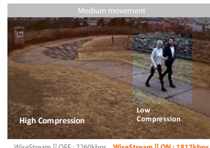
WiseStream II OFF : 7260kbps WiseStream II ON : 1817kbps
